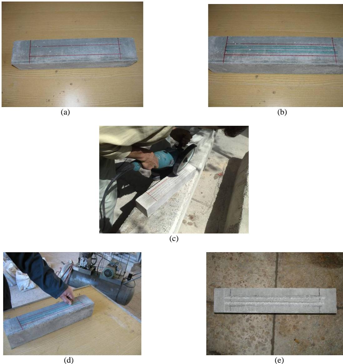
Fig. 1. Creating grooves on concrete surface
