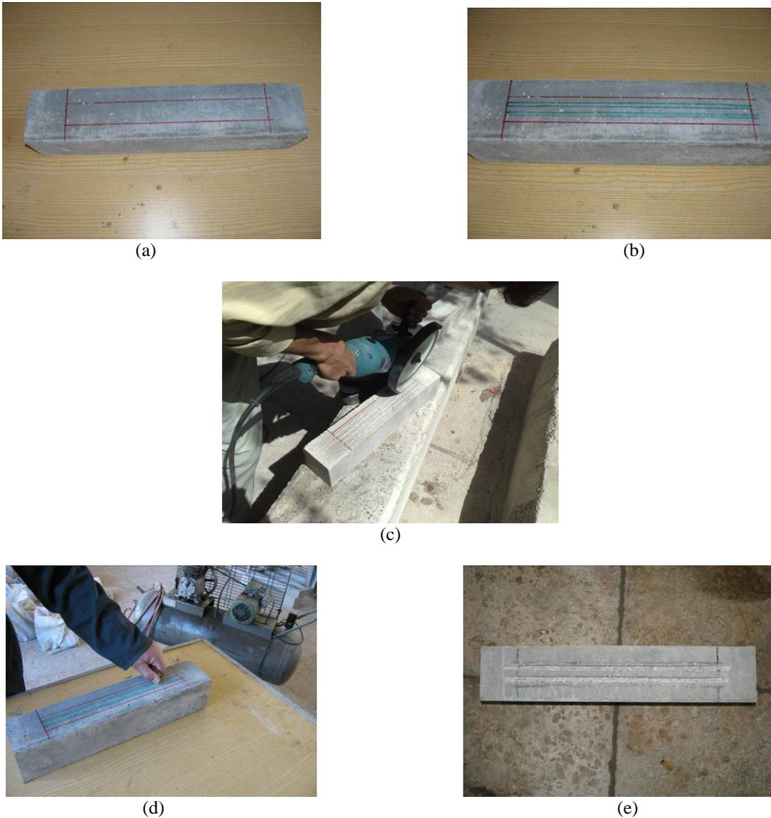
Fig. 1. Creating grooves on concrete surface
