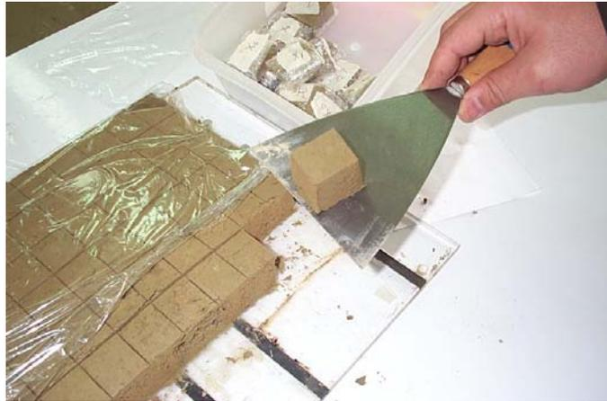
Fig. 2. Slicing the soil samples after termination of the 2-D diffusion tests
