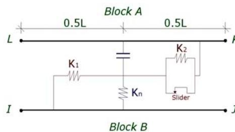
Fig. 1. The proposed joint model [8]
