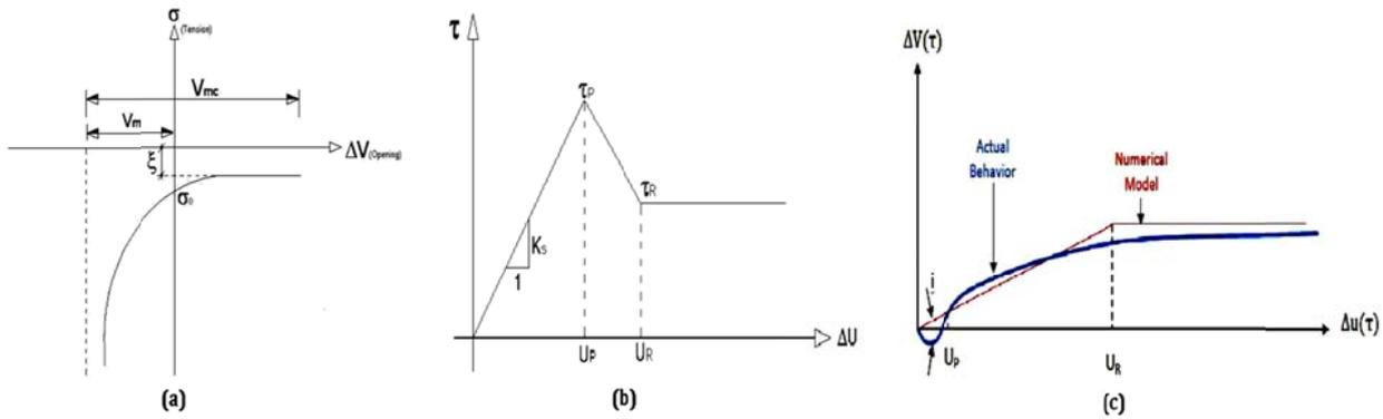
Fig. 2. Mechanical behavior of a joint element (a) Normal Behavior (b) Shear behavior (c) Dilational Behavior [10]
