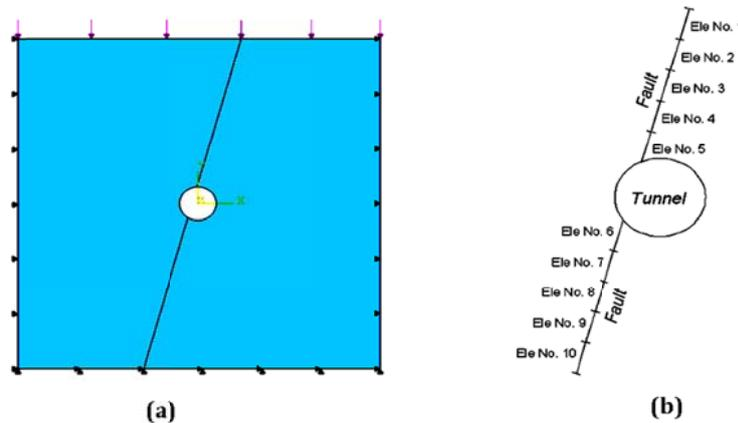
Fig. 3. (a) Fault model crossing the tunnel (b) Element numbers of the fault crossing the tunnel
