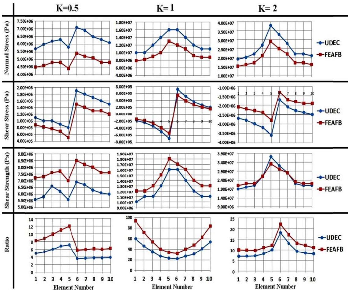
Fig. 4. Results of analyses for a fault with shear stiffness of 0.2 GPa
