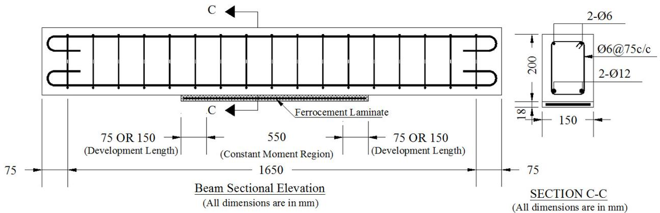
Fig. 7. Detail of beam with precast Ferrocement Laminate B (Group 'C')
