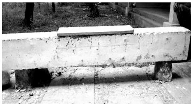
Ferrocement Laminate placed to the inverted beam
