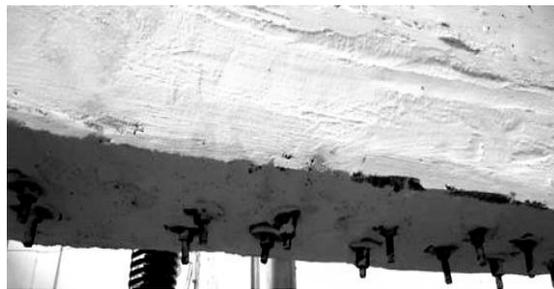
(d) Beam soffit with Ferrocement Laminate A after white wash
