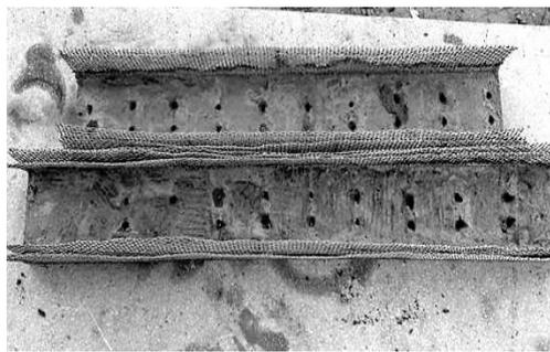
(a) Ferrocement Laminates 700 mm and 850 mm long
