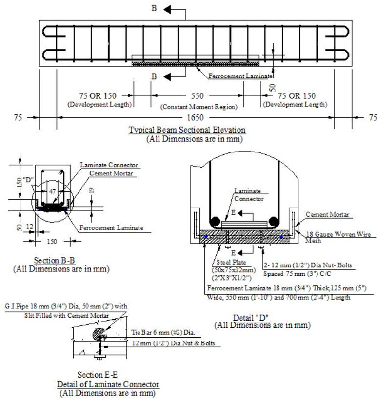
Fig. 5. Detail of beam with precast Ferrocement Laminate A (Group 'B')
