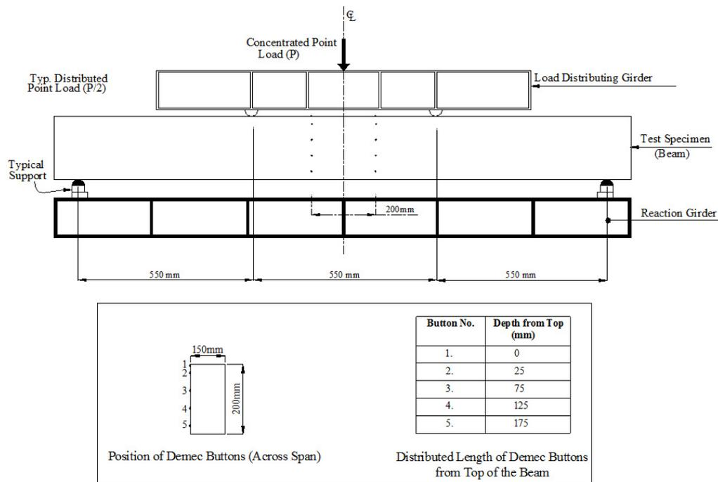
Fig. 3. Typical loading arrangement for the tested beams
