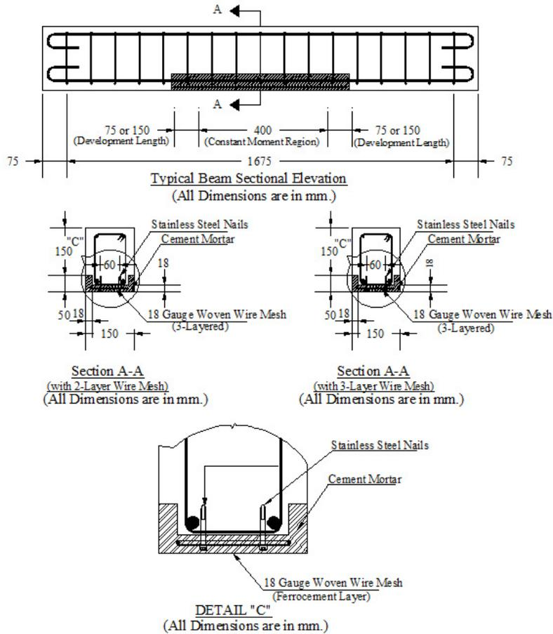
Fig. 4. Detail of beam with cast in situ Ferro-mesh layers (Group 'A')
