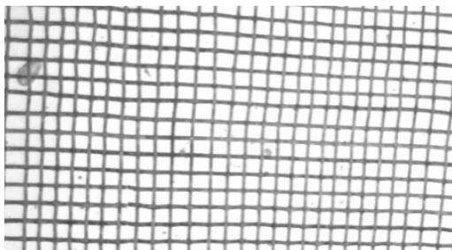
Fig. 1. Sample woven Ferro-mesh
