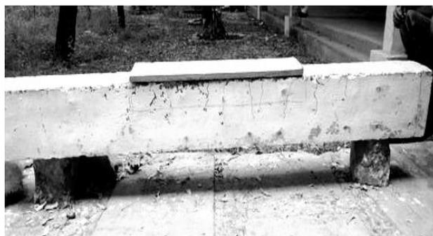
Ferrocement Laminate placed to the inverted beam
