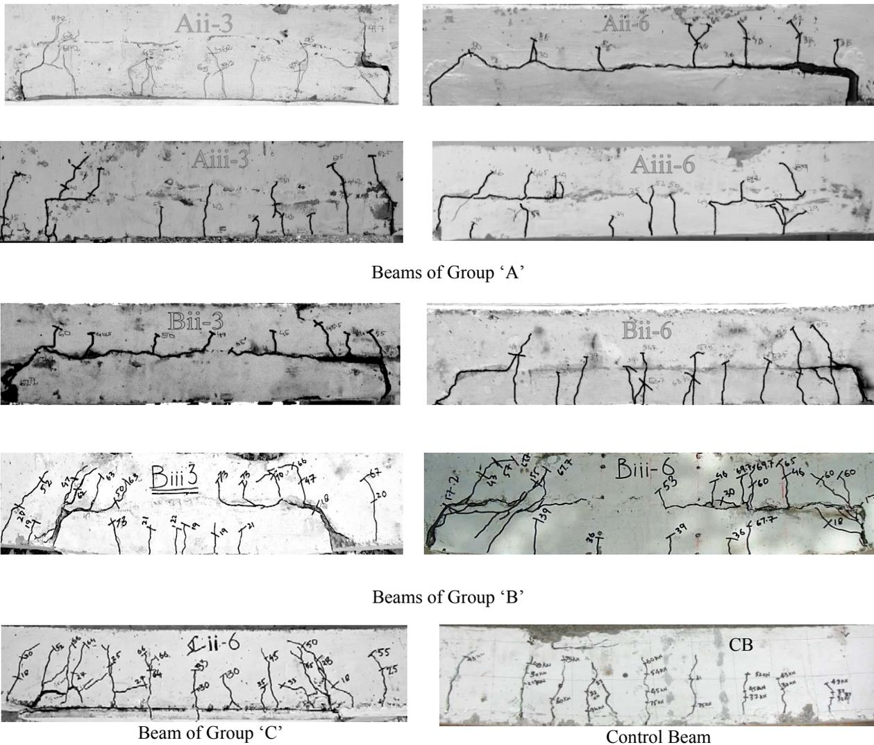
Fig. 10. Cracks pattern of beams after failure
