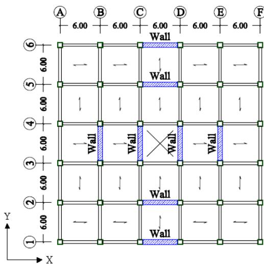
Fig. 2. The structural plan of the model A
