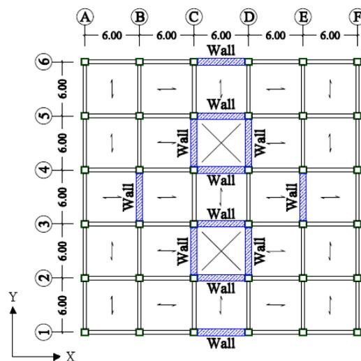
Fig. 3. The structural plan of the model B
