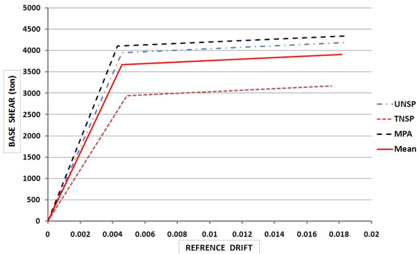
Fig. 11. The ideal bilinear diagrams of the pushover analyses for model B
