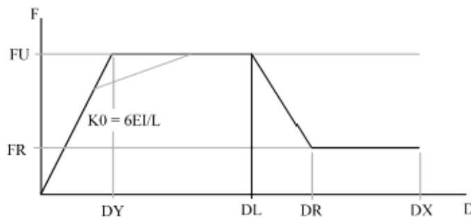
Fig. 5. Force-deformation relationship [39]
