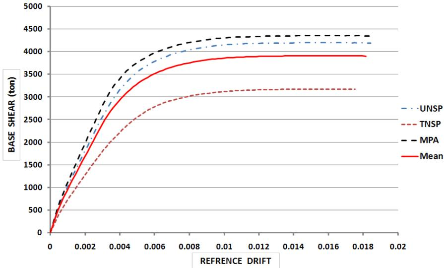
Fig. 10. The capacity curves of various pushover procedures for model B
