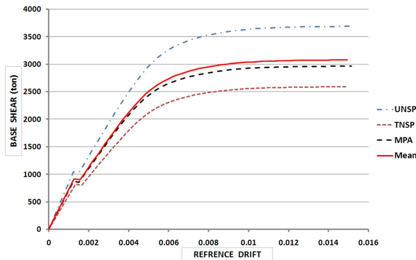
Fig. 8. The capacity curves of various pushover procedures for model A
