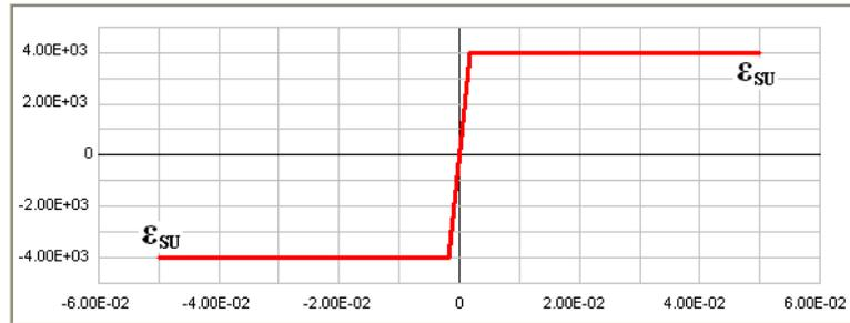
Fig. 7. Nonlinear properties of steel bar
