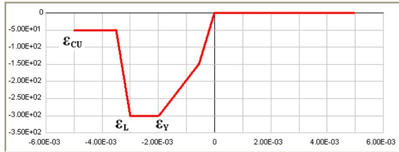
Fig. 6. Nonlinear properties of concrete material
