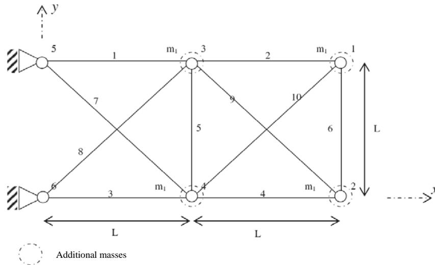
Fig. 1. 10-bar truss structure with added masses
