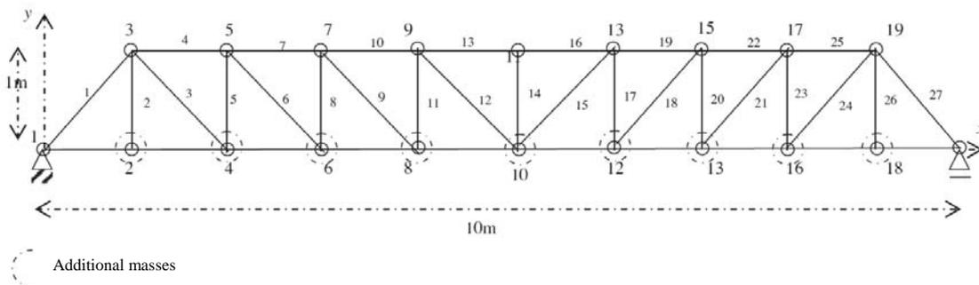
Fig. 2. Initial configuration for the 37-bar truss structure with added masses
