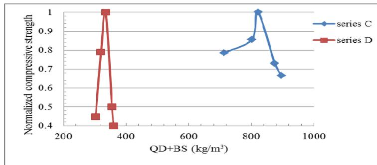
Fig. 2. Relationship between compressive strength and QD+BS
