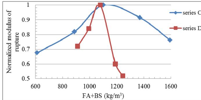
Fig. 4. Relationship between modulus of rupture and FA+BS
