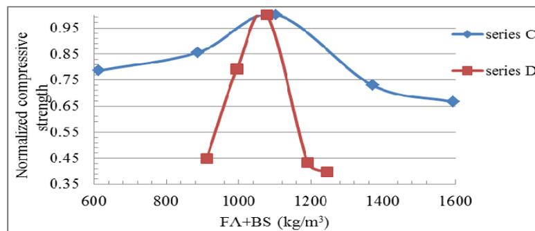
Fig. 3. Relationship between compressive strength and FA+BS
