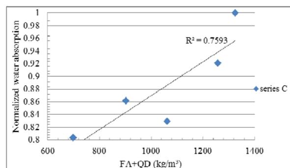
Fig. 9. Relationship between water absorption and FA+QD
