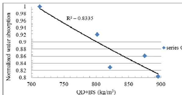
Fig. 8. Relationship between water absorption and QD+BS
