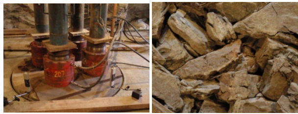
(a) Compression of soils (b) Soils after testing Fig. 4. Compression of the coarse-grained soils
