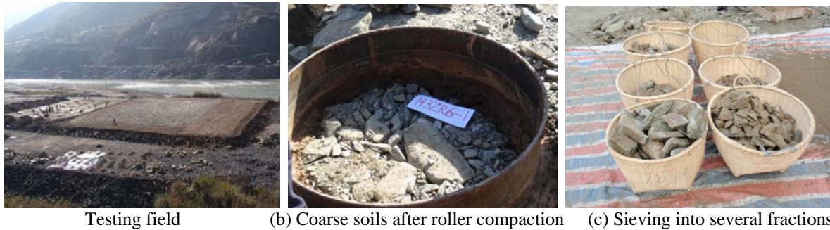
Fig. 1. Testing soils used in the oedometer tests
