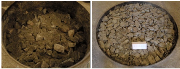
(a) Filling of the container (b) Testing specimen Fig. 3. Oedometer test specimen
