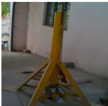
Fig. 3. Drop weight impact test setup
