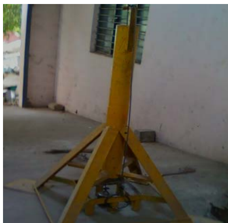
Fig. 3. Drop weight impact test setup
