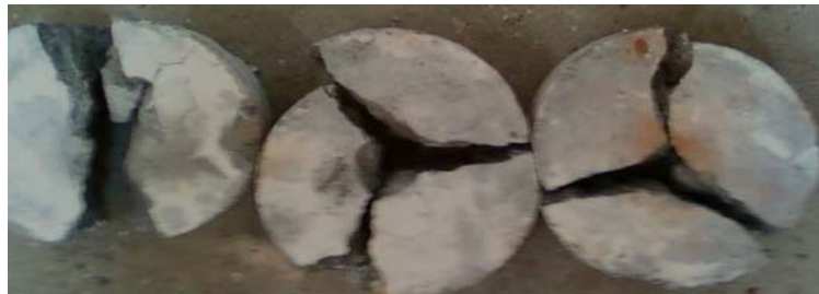
Fig. 4(b). Failure pattern of R1 specimen
