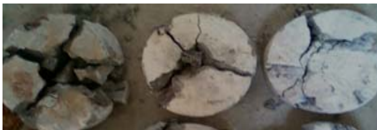
Fig. 4(d). Failure pattern of R3 specimen
