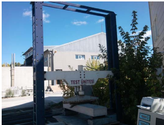
Fig. 7. Testing unit and tested beam appearance before testing
