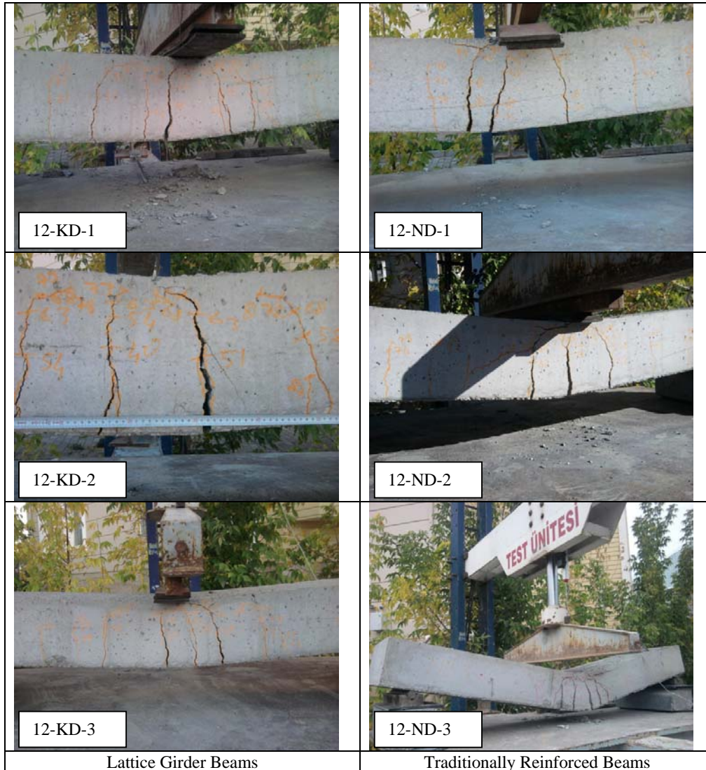
Fig. 10. Crack pattern of Type – I and Type – II beams after test
