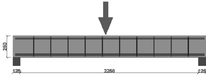
Fig. 4. Longitudinal section of tested beams (Dimensions in mm)
