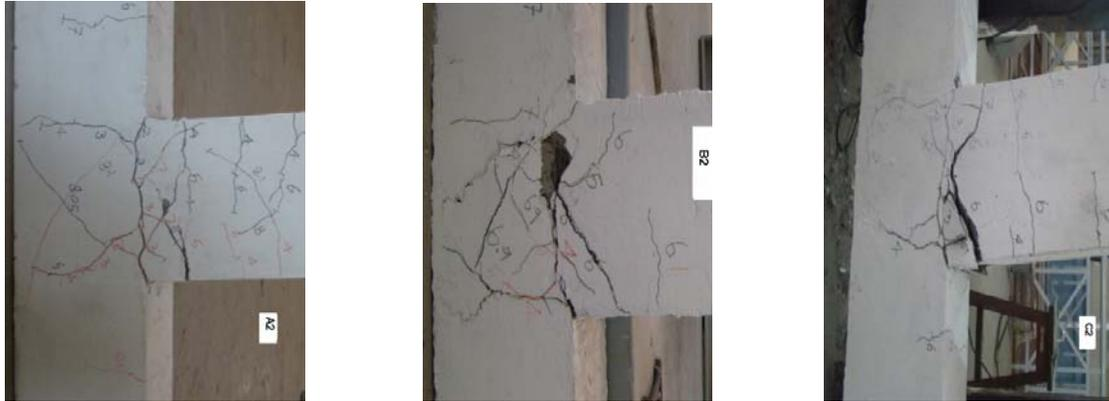
Fig. 13. Crack Pattern of Group-II (A2, B2, C2)
