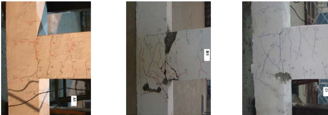
Fig. 12. Crack Pattern of Group-I (A1, B1, and C1)
