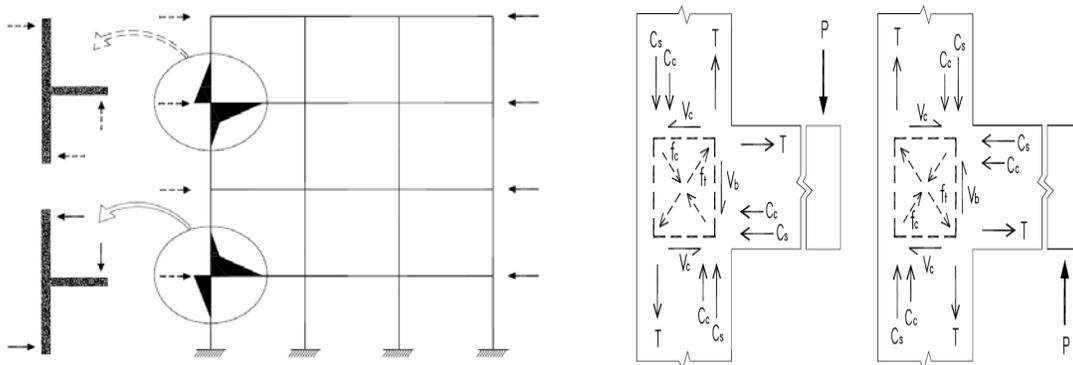
Fig. 4. Test specimen definition with forces acting on a joint core
