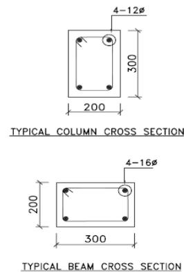
Fig. 2. Beam and Column size
