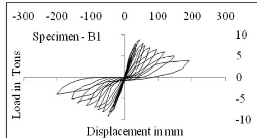
Fig. 6b. Load vs displacement
