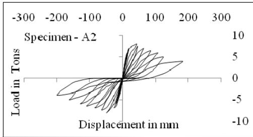
Fig. 8a. Load vs displacement
