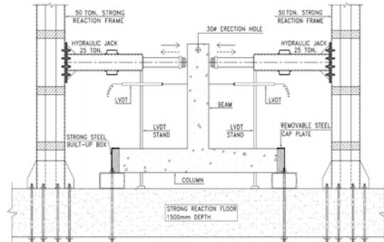
Fig. 5b. Schematic diagram of test setup
