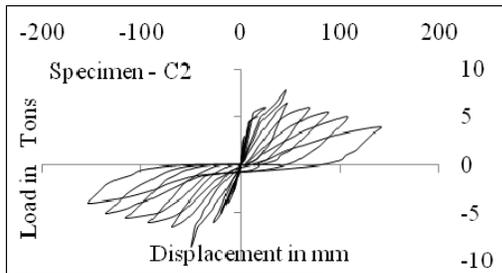
Fig. 8c. Load vs displacement
