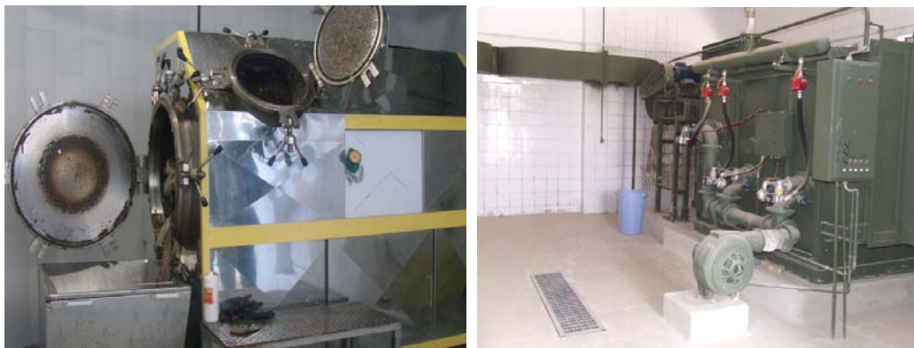
Fig. 3. Examples of autoclave equipment (left) and an incinerator (right)
