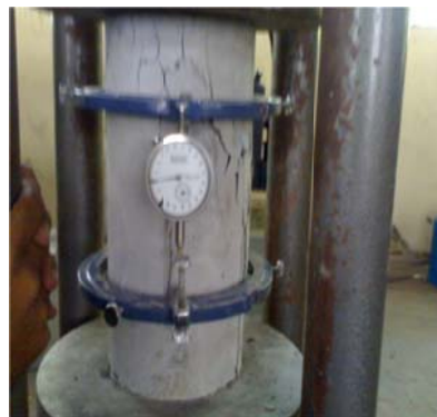
Fig. 2. Compressometer test for chord modulus of elasticity
