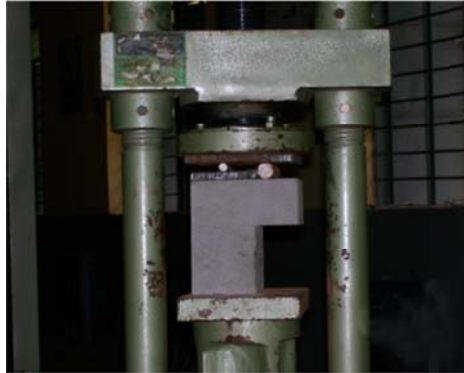
Fig. 3. Shear test on 'L' Specimen
