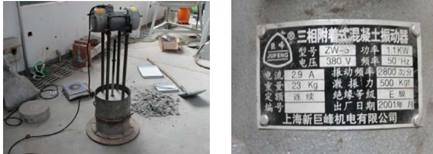
Fig. 12. The equipment used in the maximum density test
