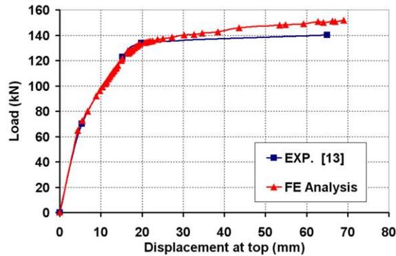
Fig. 4. Comparison of experimental and FE analysis envelope curves for wall RW1 tested by Thomsen and Wallace [13]
