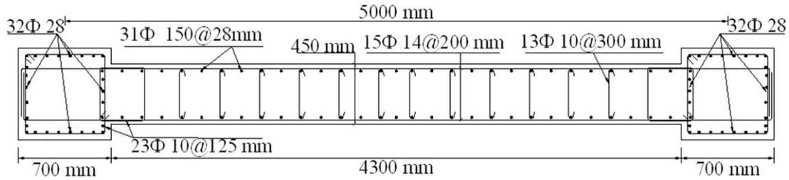
Fig. 5. Section properties of the shear wall SH3
