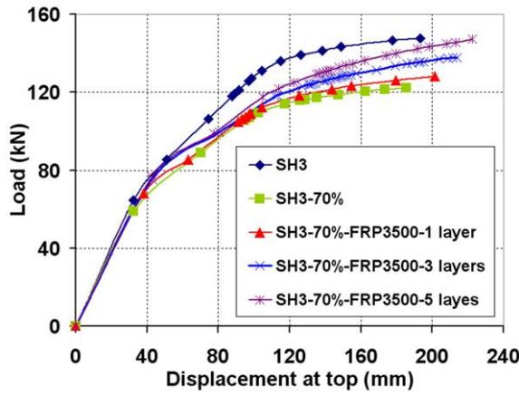
Fig. 8. Effect of number of FRP sheet layers at wall boundary elements in specimen SH3-b70%
