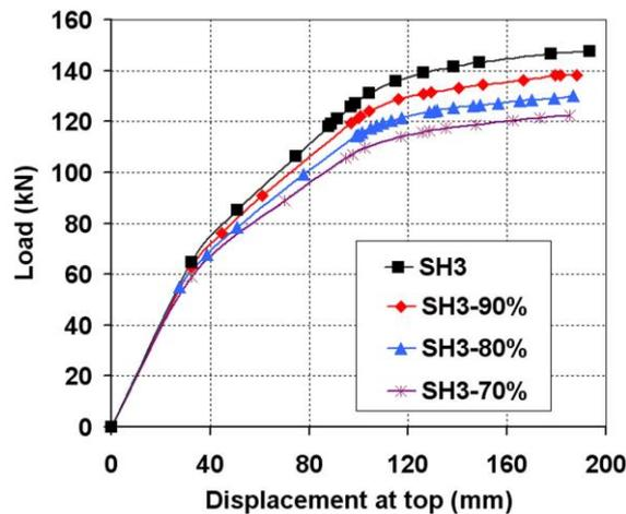
Fig. 6. Effect of wall boundary elements longitudinal steels reduction in specimen SH3
