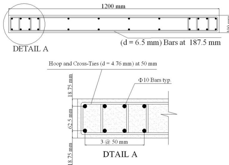
Fig. 2. The detail of the specimen RW1 tested by Thomsen and Wallace [13]
