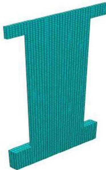
Fig. 3. The meshed model of wall tested by Thomsen and Wallace
