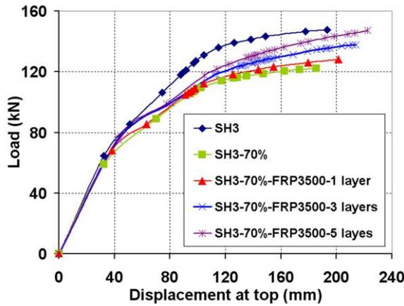
Fig. 8. Effect of number of FRP sheet layers at wall boundary elements in specimen SH3-b70%
