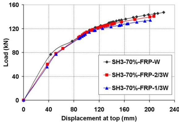
Fig. 9. Effect of FRP sheet width reduction at wall boundary elements in specimen SH3-b70%
