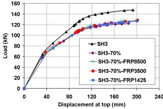
Fig. 7. Effect of wall height in which boundary elements are strengthened with FRP sheet in specimen SH3-b70%
