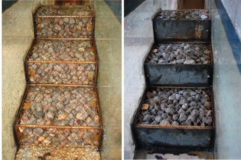
Fig. 3. Two gabion stepped spillways with a slope of 1:2, without (left) and with (right) vertical impervious plates
