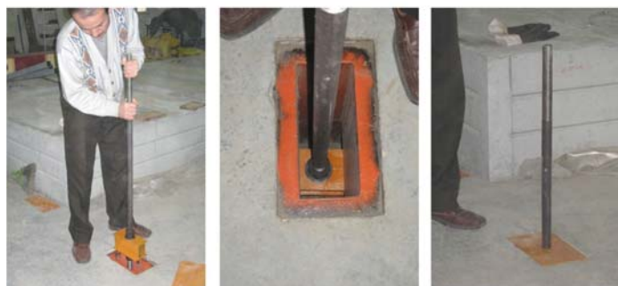
Fig. 4. Details and usage of the anchorage system
