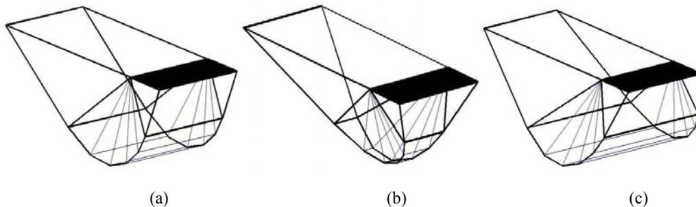
Fig. 5. The inclination of lateral failure surfaces in three dimensional space, a) zero value for  $\theta_1$  and  $\theta_2$  (vertical), b) negative value (inclined inward), c) positive value (inclined outward)
