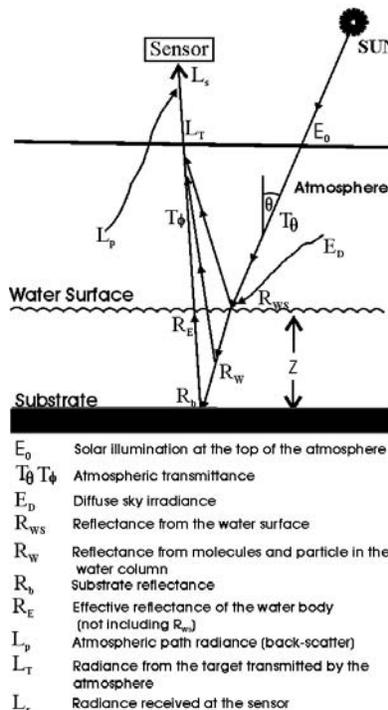
Fig. 3. Radiance path and factors influencing the amount of radiance reaching a sensor over a water-mass [1]
