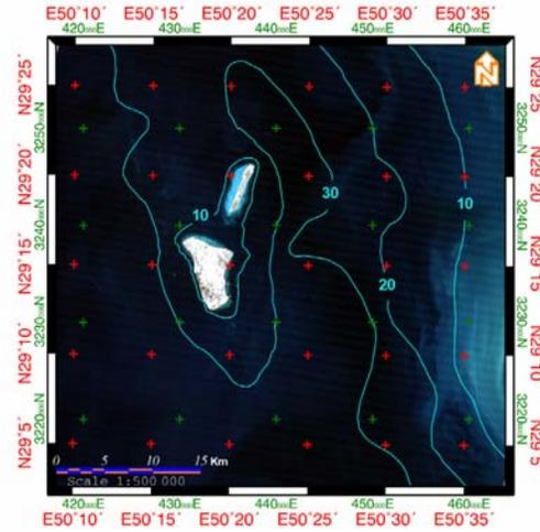
Fig. 2. Bathymetry contour lines overlaid on Landsat TM image of study area, depths are in meter, image display 321: (RGB) [ Landsat TM index 164/40, 1998]
