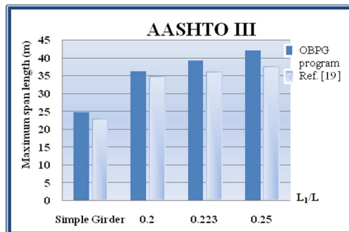
Fig. 9. Comparison of the optimization of simple and spliced girders for the AASHTO III section
