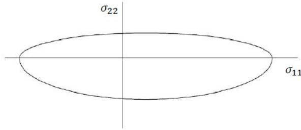
Fig. 4. Tsai-Wu failure envelope ( $I_F = 1.0, F_{12} = 0.0$ )
