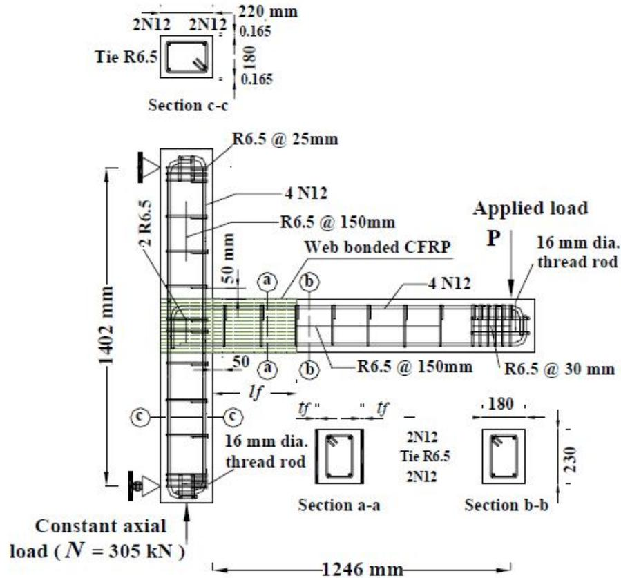
Fig. 2. Details of the selected joint [18]
