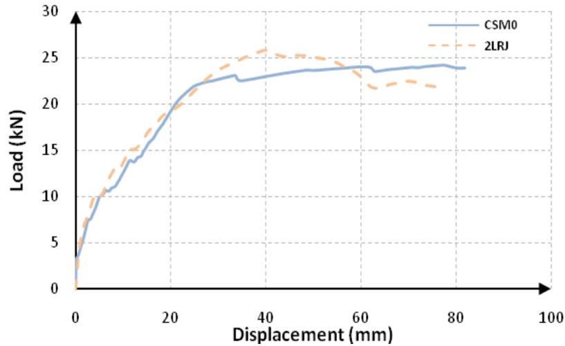
Fig. 10. Load-deflection curve of original and retrofitted joint
