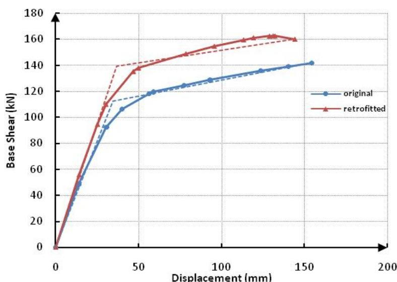
Fig. 12. Base shear-root displacement relationship of original and retrofitted specimen
