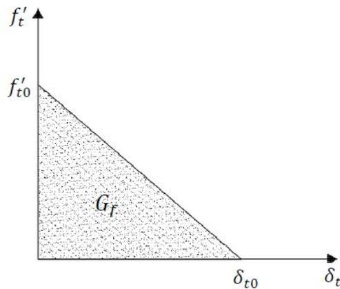
Fig. 7. The concrete tension softening
