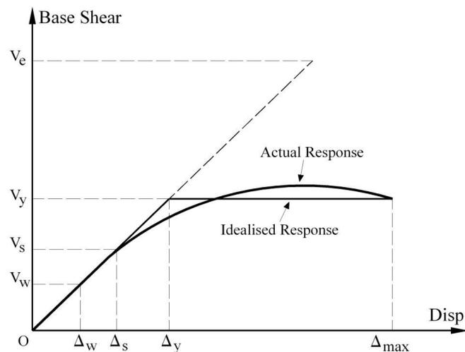
Fig. 13. Idealised bi-linear model of the pushover curve for calculation of earthquake response parameters
