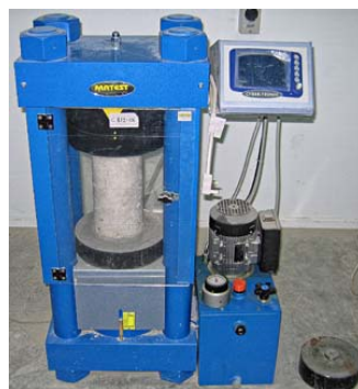
Fig. 1. Testing setup for measuring the compressive strength of concrete
