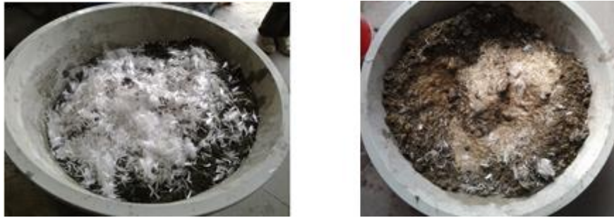
Fig. 2. Polypropylene and steel fiber additives used in plasters
