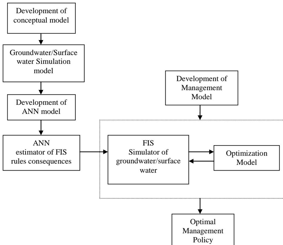
Fig. 4. Schematic representation of the linked simulation-optimization model
