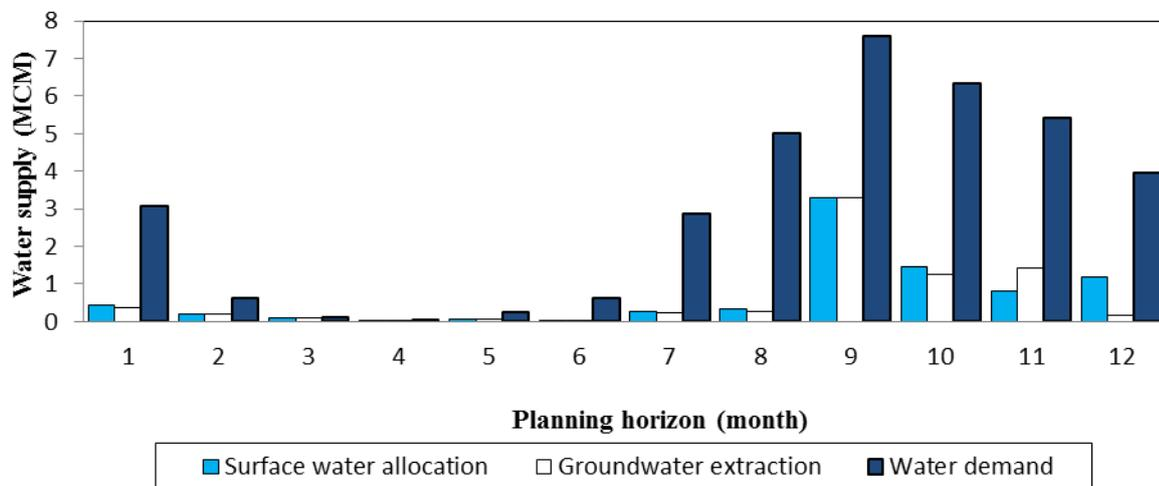
Fig. 5. The water demand and monthly allocated surface water and groundwater to Khamiran zone
