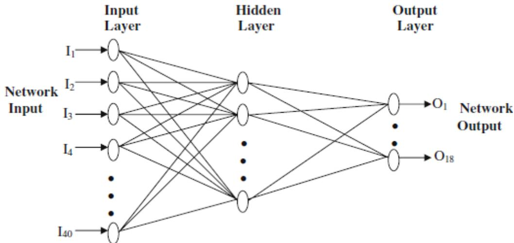
Fig. 3. Three-layer LMBP neural network architecture
