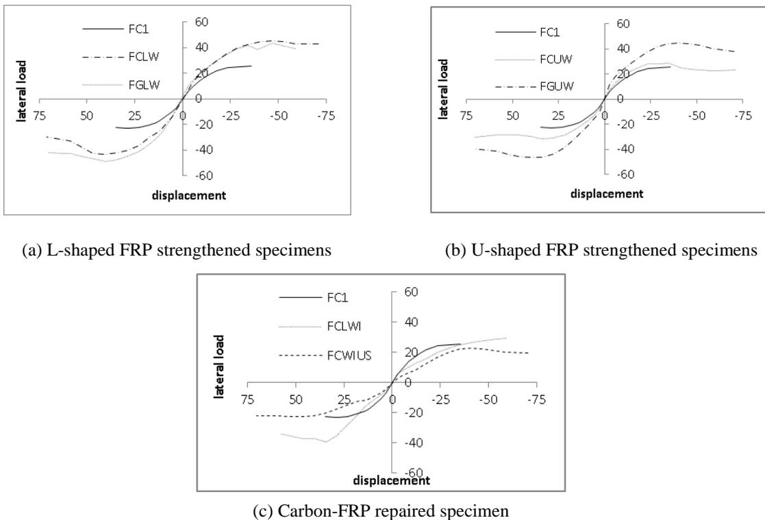
Fig. 7. Lateral load-displacement skeleton curves
