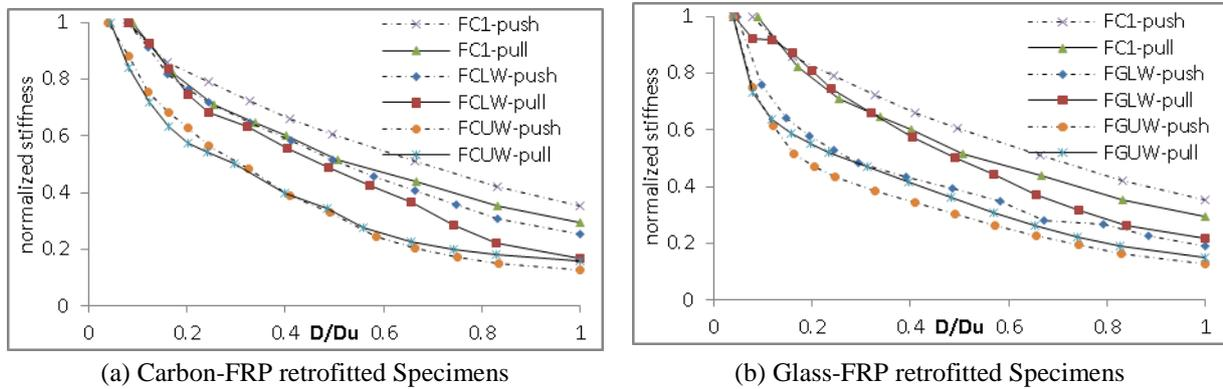
Fig. 8. Curves of normalized-stiffness versus normalized-displacement
