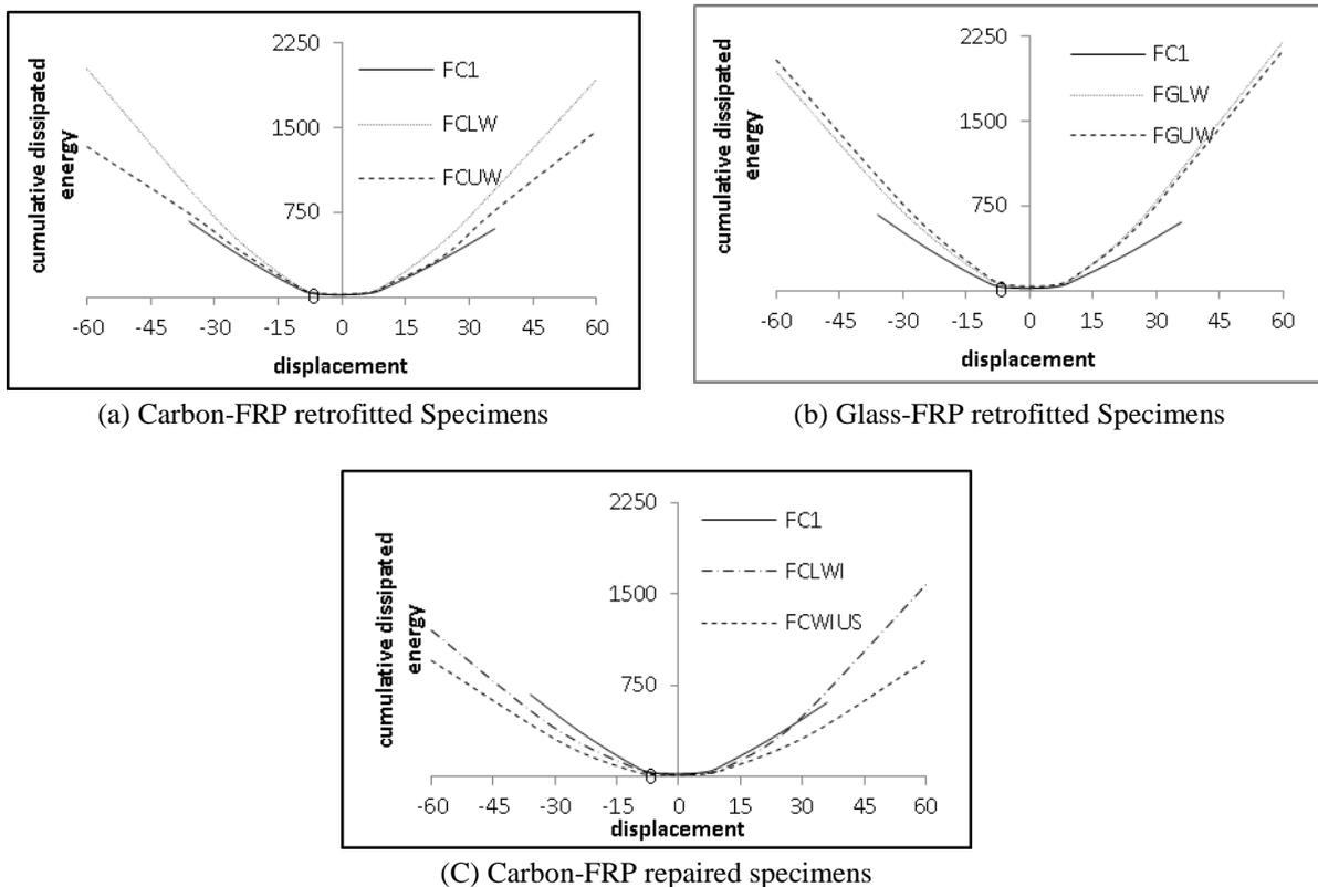
Fig. 9. Curves of energy dissipation versus displacement
