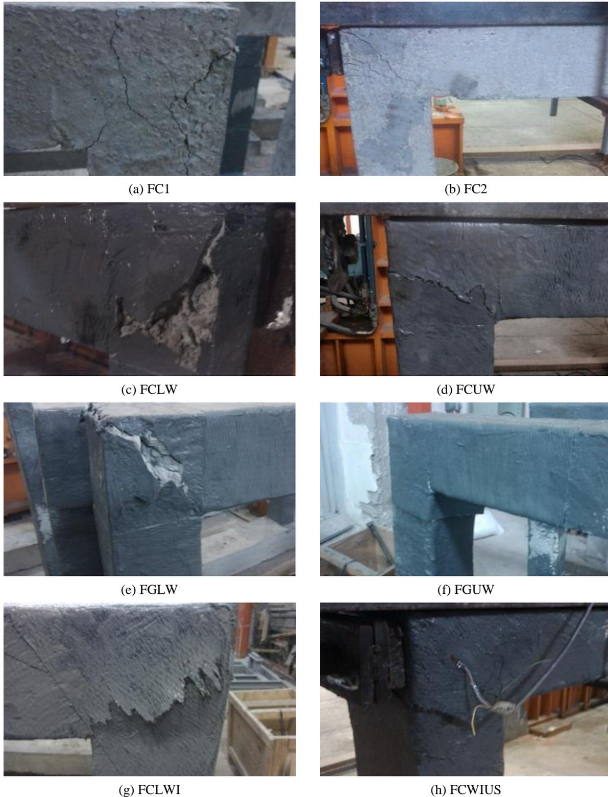
Fig. 5. Damage patterns of specimens
