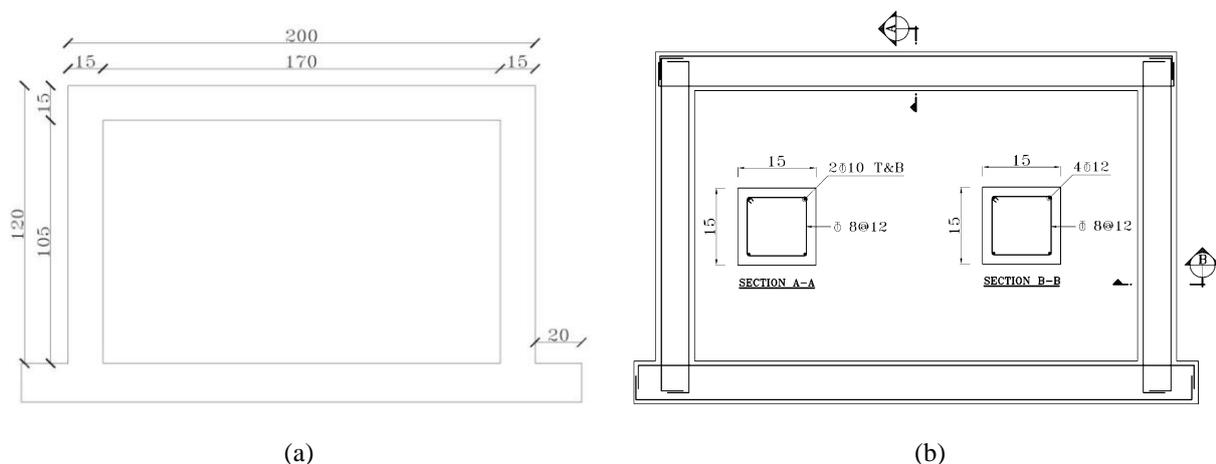
Fig. 1. Dimension and reinforcement of tested frame
