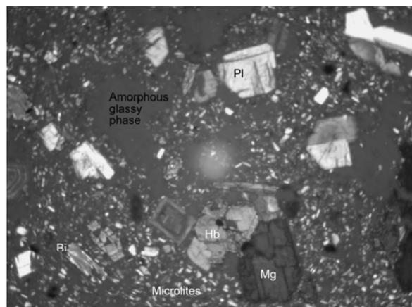
Fig. 2. Microscopic observations under polarized light (x4, XPL). Hyalo microlitic porphyric texture with phenocrysts/microphenocrysts of plagioclase (Pl), hornblende (Hb), biotite (Bi) and magnetite (Mg) as an opaque phase in a fine-grained glassy groundmass
