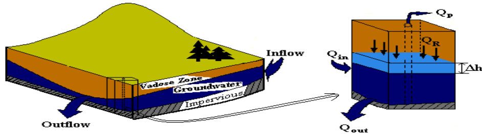
Fig. 8. Schematic of ground water balance used in CRD method
