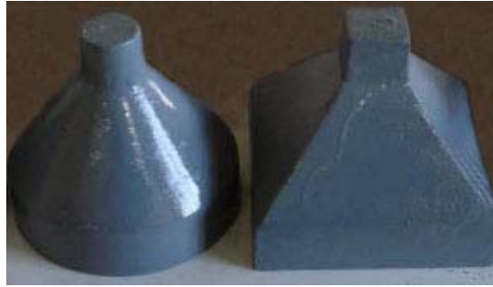
Fig. 2. Conical and pyramidal shell foundations constructed with cast iron for axisymmetric and three-dimensional test conditions
