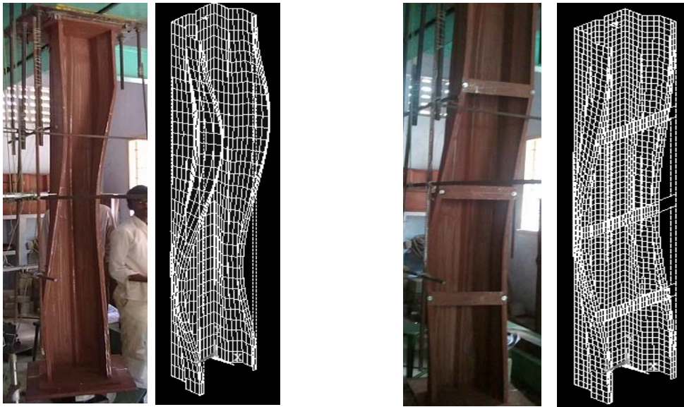
Fig. 7. Deformed shape of RC-SO
