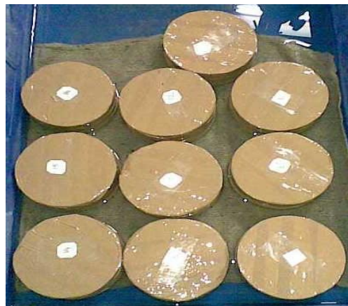
Fig. 3. RAC Specimens under Sorptivity testing
