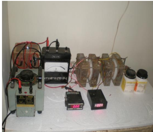
Fig. 5. RAC Specimens under RCPT testing
