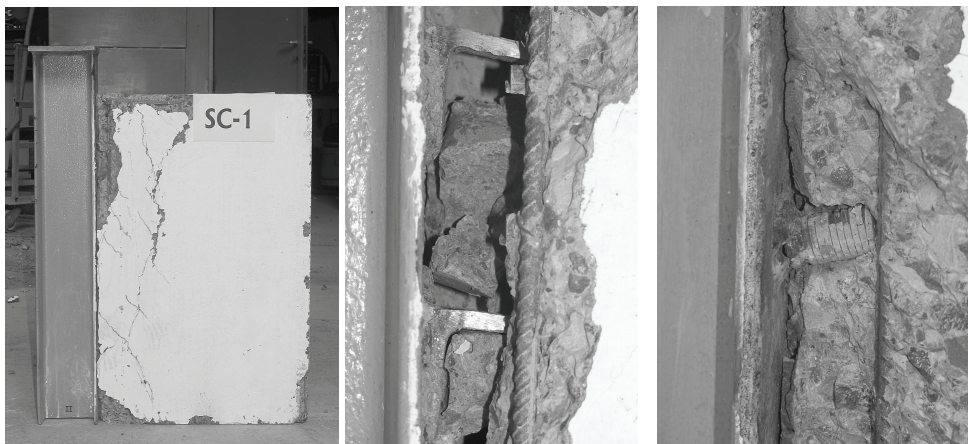
Fig. 3. Types of failure for some test samples
