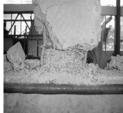
Fig. 6. Observed failure mechanism of specimen CSC1 [12]
