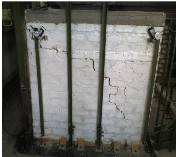
Fig. 6. Mode of failure of the wall NWFS
