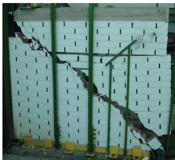
Fig. 4. Mode of failure of the wall SWES
