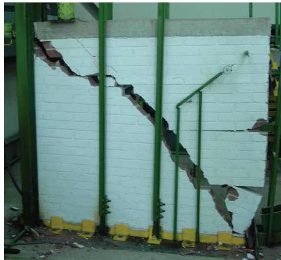
Fig. 3. Mode of failure of the wall SWFS
