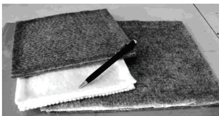
Fig. 1. A picture view of the types (A) and (B) E-GCLs fabricated in the laboratory
