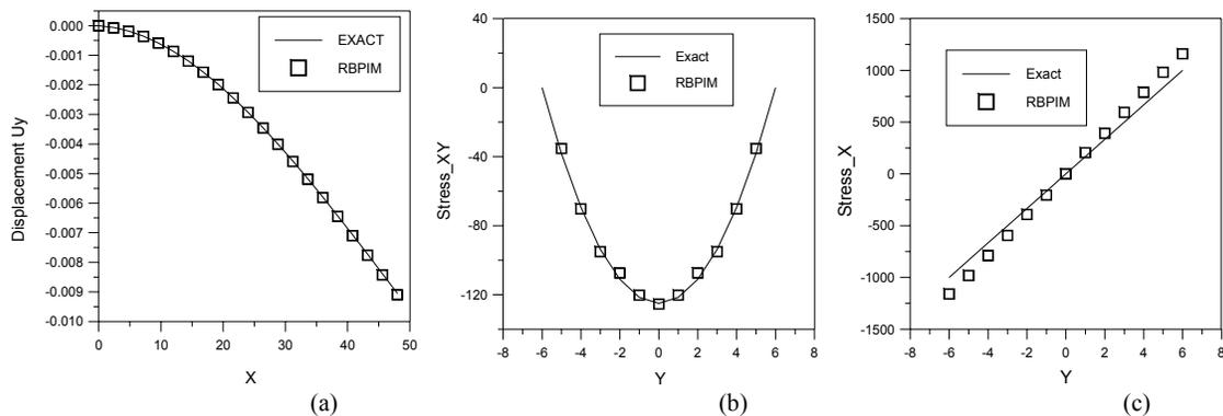
Fig. 2. Comparison between the exact solution results and RBPIM results for a) deflection b) stress\_xy c) stress\_x
